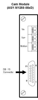
Connect terminals to Main terminal block when required. ONLY one CAM module may be connected.
